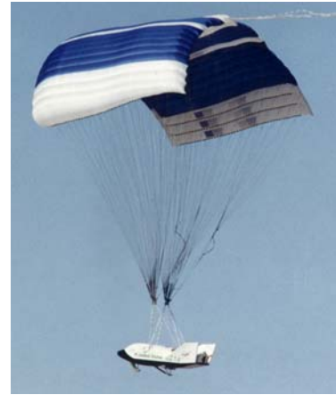
Figure 17 - X-38 prototype V-132 during the fifth drop test at Edwards, March 2000.
