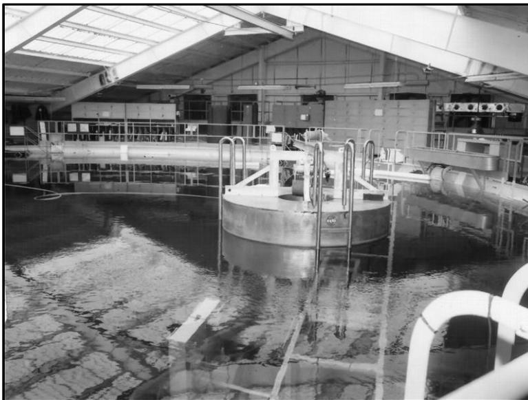
**Figure 2. The Neutral Buoyancy Simulator (NBS) at Marshall Spaceflight Center (MSFC)(photo courtesy of NASA).**
